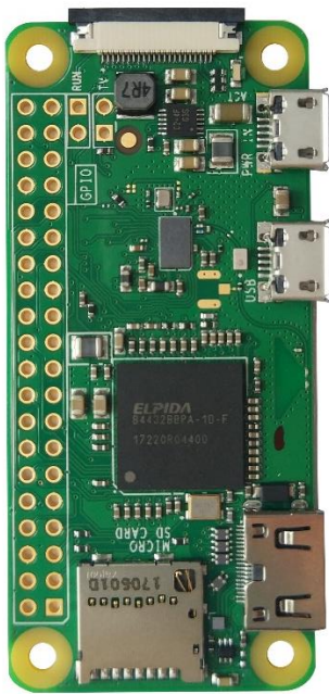
Practicality picture of Raspberry Pi Zero:
