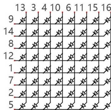
Connection mode of Common Cathode
