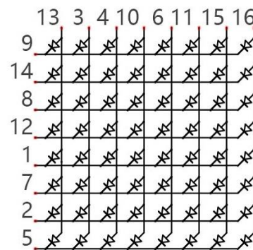
Connection mode of Common Cathode
